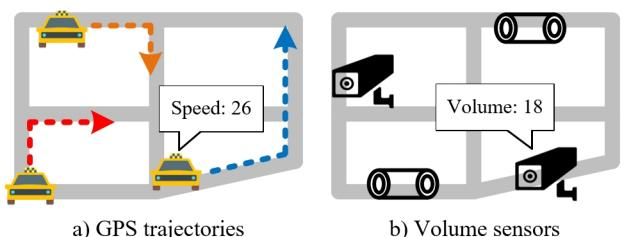
Figure 1: Traffic speed and volume sensors
